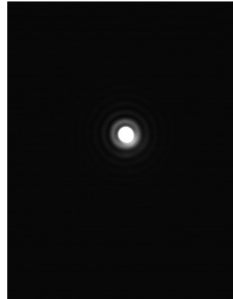
Airy disk deformed by speckle noise
